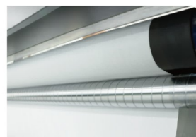
Rubber roll media feeding system, more suitable for thin paper printing
