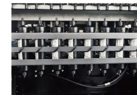
Air degassing unit removes micro bubbles in ink while transferring ink to main ink tank
