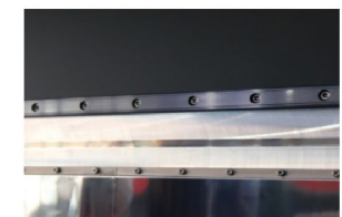
high stability magnetic encoder strip
